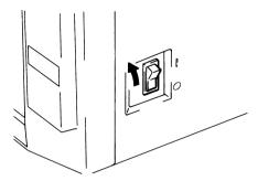
Press the Power Switch of the printer to the I (ON) position.
